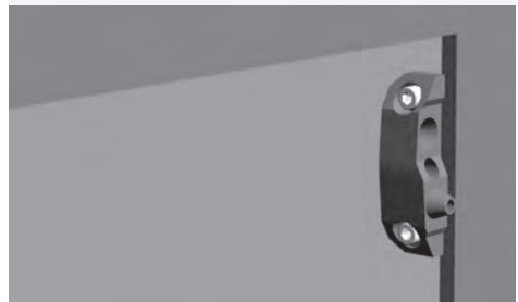
Fig. 12 – sections connection (connectors + M8 screw)
