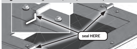
Fig. 26 – sealing of roof parts (PU sealant) -F
