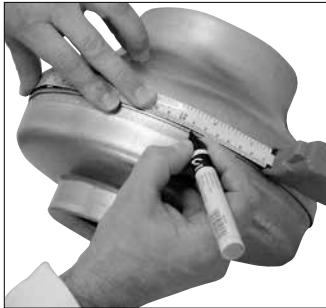
1. Mark the measure of **B** on the fan for the placement of the mounting brackets.
