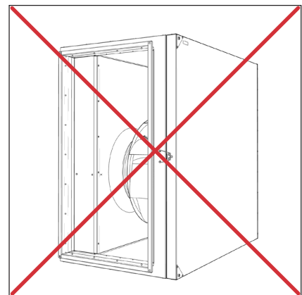
Installed with lid facing to the side.
