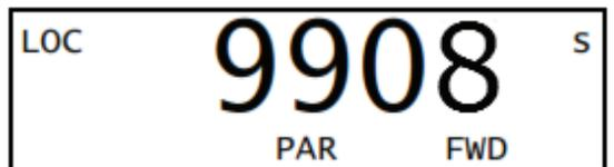
Setup the motor's rated power consumption as indicated on the motor label. For example 4Kw
