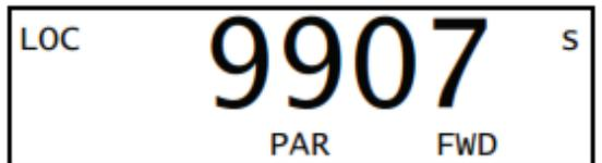
Setup the motor's rated speed as indicated on the motor label. For example. 2830 rpm
