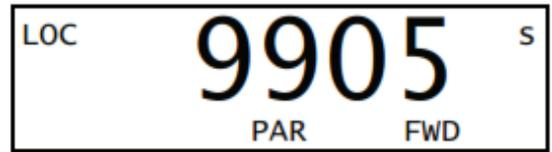
Setup the motor's rated current as indicated on the motor label. For example 2,6A
