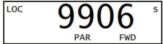
Setup the motor's rated frequency as indicated on the motor label. For example 50Hz
