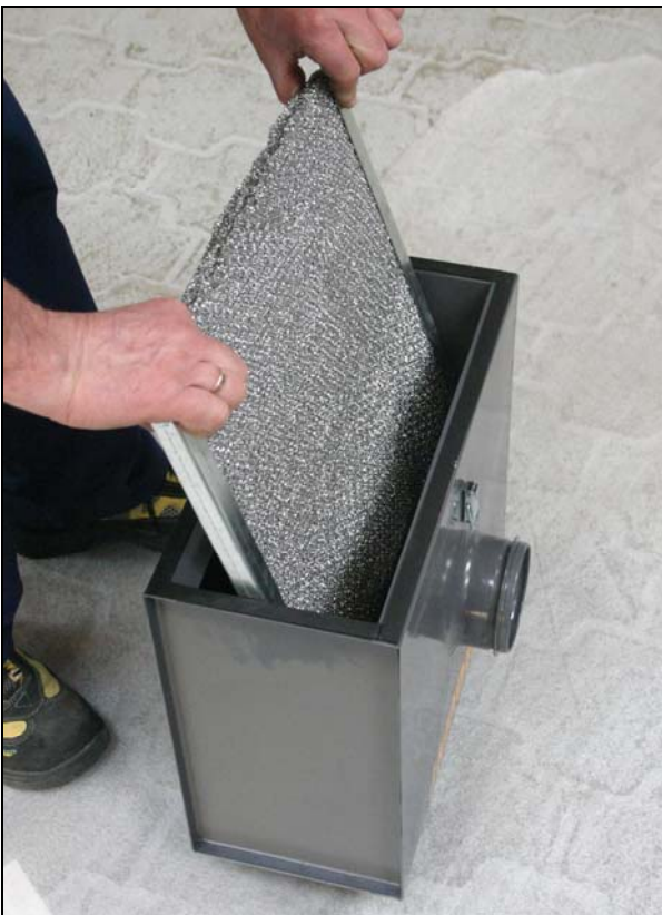
Pull up the filter/alumesh
