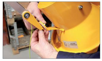
4. Now mount the hood on the outer joint by putting the supplied 8mm bolt though 3 spring washers, the hood bracket, the friction disc and secure with an 8mm lock nut.
