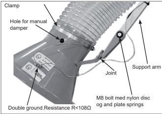
When installing 4 meter extraction arm, 2 joints, first mount inner arm, then the middle and finally the outer
