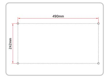
Hole positioning for attachment of cabinet
