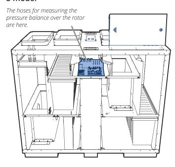
Connect the pressure gauge with the –hose to A (blue hose in the unit) and the +hose to B (red hose in the unit). Run the unit at the correct operating point for the system in question.
