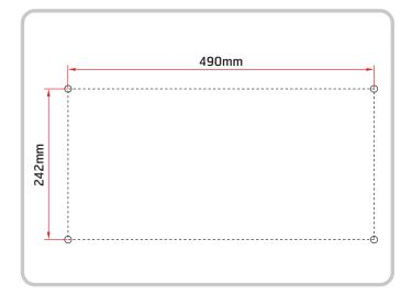
Hole positioning for attachment of cabinet
