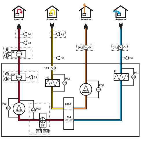
The unit can only have one heating battery - water or electric.
