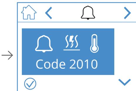
The alarm is displayed in different places on the different screens. Press the alarm icon to access the alarm handling menu.
