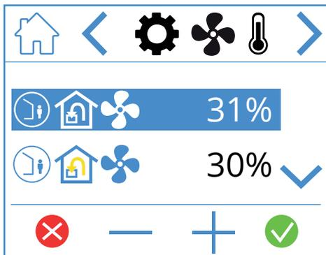
To adjust a value, highlight the line you want to change by pressing it so that the line turns blue. Then press – or + to decrease or increase the fan setting. When you reach the desired value, press to confirm. The value is written to the unit and the fan changes speed.
