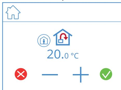
You change the temperature from the home screen. There you press the symbol for temperature or degrees. A new screen will open. Press - or + to decrease or increase the temperature. To confirm, press . To undo the change, press . The panel will then return to the home screen.
