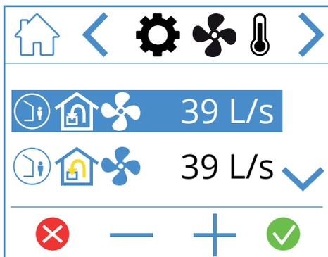
To adjust a value, highlight the line you want to change by pressing it so that the line turns blue. Then press – or + to decrease or increase the fan setting. When you reach the desired value, press to confirm. The value is written to the unit and the fan changes speed. To cancel and not change the value, press . The same procedure applies to changing the temperature mode.
