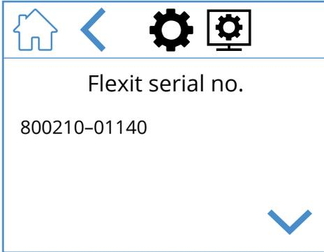
For info only. Shows hardware and software version on the panel and serial number on the unit. Press HOME to go to the selected home screen.
