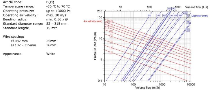
The **PVC White** fulfills all the requirements and are classified as specified within EN 13180: Ventilation for buildings – Ductwork - Dimensions and mechanical requirements for flexible ducts.
