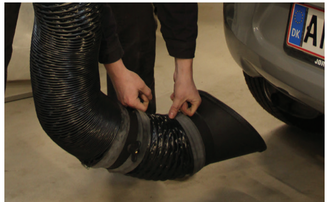
Mount the nozzle with M6 x 25 insex screws with washer. Use a size 5 Allen key.
