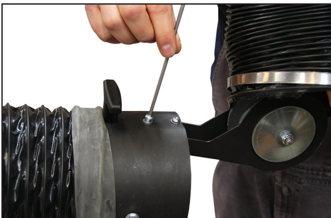
Mount the nozzle with M6 x 25 insex screws with washer. Use a size 5 Allen key.
