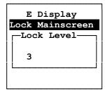
To set the lock level, go to "Control Menu", "Settings", "E Display" then "Lock Mainscreen". Select level using  $[\ \ \ ]$  and  $[\ \ \ \ ]$ , confirm by pressing  $[\ \ \ \ \ ]$ . Press [ESC] to return to the Control Menu.
