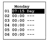
Use  $[\mathring{1}]$  and  $[\mathring{4}]$  to set the hour and confirm by pressing  $[\mathscr{J}]$ . Now set the minutes using  $[\mathring{1}]$  and  $[\mathring{4}]$ , confirm by pressing  $[\mathscr{J}]$ . Finally, set the operating mode using  $[\mathring{1}]$  and  $[\mathring{4}]$ , confirm by pressing  $[\mathscr{J}]$ . Press [ESC] twice to return to Control Menu. To reset all calendar settings, see section 2.5.5.5.
