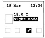
To select Night Mode go to "Control Menu" and select "Mode start/stop". Use  $[\hat{U}]$  and  $[\mathcal{V}]$  to mark up "Night mode" and confirm by pressing  $[\mathcal{V}]$ .
