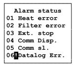
To access the alarm status go to "Control Menu" and select "Alarm menu". Active alarms will be marked "!". Browse the pages using [♠] or exit the menu by pressing [ESC].
