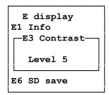
To change the contrast go to "Control Menu", "Settings" select "E Display" then "E3 Contrast". Set contrast level using  $[\ \ \ ]$  and  $[\ \ \ \ ]$ , confirm by pressing  $[\ \ \ \ \ ]$ . Press [ESC] to return to the Control Menu.
