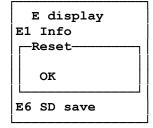
To restore factory settings go to "Control Menu", "Settings", "E Display" and select "E4 Fact. Sett.". Confirm by pressing [₺] twice or cancel by pressing [ESC].
