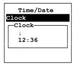
To set the clock go to "Control Menu" select "Time/Date" and then "Clock". Set the hours using  $[\ \ \ \ ]$  and  $[\ \ \ \ ]$ , confirm by pressing  $[\ \ \ \ \ ]$ . Set the minutes using  $[\ \ \ \ \ ]$  and  $[\ \ \ \ \ ]$ , confirm by pressing  $[\ \ \ \ \ \ \ ]$ . Press [ESC] to return to Control Menu.
