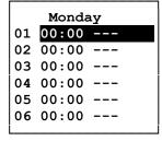
To set the calendar go to "Control Menu" and select "Calendar". Use  $[\mathring{1}]$  and  $[\mathring{4}]$  to mark up the day to modify and confirm by pressing  $[\rlap/{e}]$ . Now use  $[\mathring{1}]$  and  $[\rlap/{4}]$  to mark up the setting to modify and confirm by pressing  $[\rlap/{e}]$ . Exit any time by pressing [ESC].
