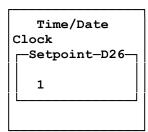
To set DST (Daylight Saving Time) go to "Control Menu", "Time/Date" and then "DST OFF/ON". Set value to 0 (OFF) or 1 (ON) using  $[\ \ \ \ \ ]$  and  $[\ \ \ \ \ \ ]$ , confirm by pressing  $[\ \ \ \ \ \ \ \ ]$ . Press [ESC] to return to Control Menu.
