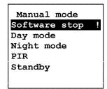
To activate this function go to "Control Menu", select "Mode start/stop" and the select "Software stop". An exclamation mark displayed after the text will indicate that this function is active.
