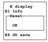
To reset the calendar go to "Control Menu", "Settings", "E Display" and select "Cal. reset". Confirm by pressing [♥] twice or cancel by pressing [ESC].
