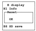
To save the logged data to the SD card go to "Control Menu", "E Display" select "E6 SD save". Confirm by pressing [ $\checkmark$ ] twice or cancel by pressing [ESC].
