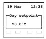
To set the desired supply air temperatures, first press [ESC]. Next, mark up the day or night setpoint using  $[\hat{\psi}]$  and  $[\hat{\psi}]$  and confirm by pressing  $[\mathcal{J}]$ . Now set the desired temperature using  $[\hat{\psi}]$  and  $[\hat{\psi}]$ . Finally, confirm by pressing  $[\mathcal{J}]$ . If this function is passcode protected, see section 1.5.0.
