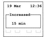
To activate Forced Mode press  $[\hat{u}]$ . The symbol  $[\mathbb{Z}]$  (0-100%) will be replaced by  $[\mathbb{Z}]$  (100%+) to indicate that Forced Mode is active. The unit will now work in Forced Mode for the preset period of time or until  $[\hat{u}]$  is pressed again.
