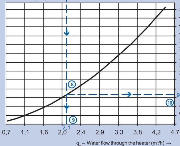
$\Delta p_w$  – Water pressure loss at water side (kPa) →
