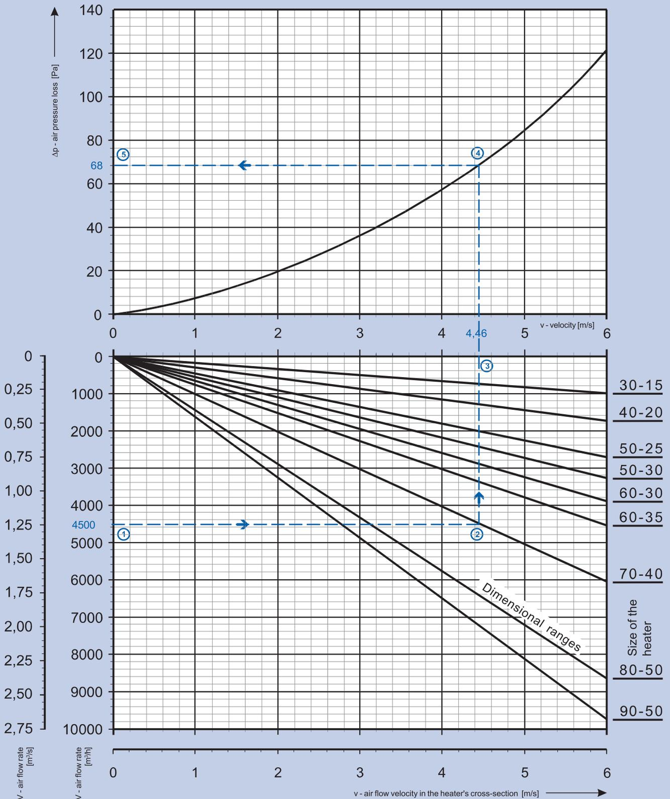
The nomogram of pressure losses is valid for all VO heaters. For the selected air flow rate ①, the air flow velocity ③ in the free heater's cross-section ②, can be read in the lower graph, and then the corresponding heater's air pressure loss ④ at the known velocity can be determined in the upper part ⑤.
