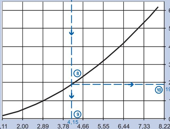
$\Delta p_w$  – Water pressure loss at water side (kPa) →
