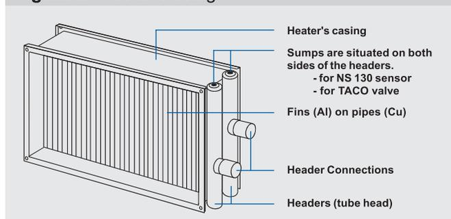
change surface is created by 0.1 mm thick aluminium overlapping fins pulled on copper pipes of  $\dot{C}$  9.52 mm (3/8"). As standard, VO heaters are manufactured in two-row versions with shifted geometry (ST 25 x 22 mm). All used materials are carefully checked so they ensure long service life and reliability. All heaters are tested under water for leakage using pressurised air of 2 MPa for five minutes.
