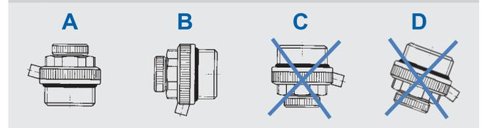
■ The TACO air-venting valves must be installed as shown in figure #13, i.e. vertically (upright) with their heads up - view A, or horizontally - view - B; in no case downwards or slanted with their heads down - C, D.
