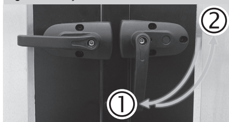
Figure 4 – Safety door lock
