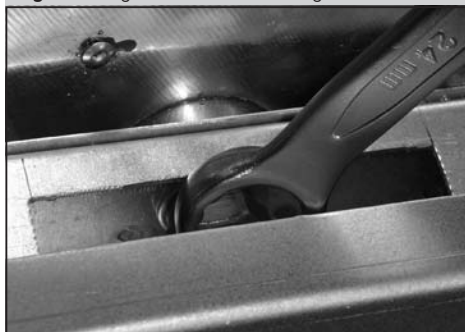
Figure 7 – Tighten the shaft bolt using wrench # 24
