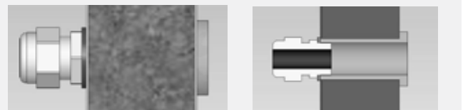
Figure 22 – cable wiring grommet design
