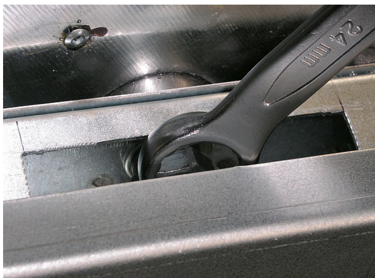
Figure 7: Tighten the shaft bolt using wrench # 24
