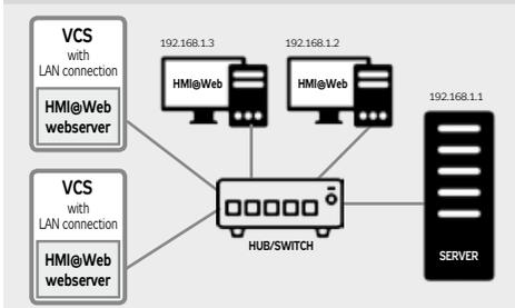
To enable HMI@Web control, it is necessary to set a unique IP address on the VCS controller within the address range of the specific network. Please refer to the figure and set the IP address under the "► LAN Connection" section (as described in step 4: Activation).
