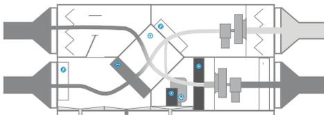
**In cases of increased humidity**, the unit transitions to a state similar to the energy-saving mode during maximum dehumidification (2nd stage of dehumidification).
