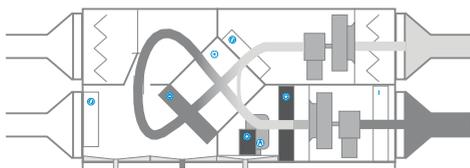
**In cases of increased humidity in the space**, the recirculation damper closes. Depending on the humidity in the exhaust, the proportion of fresh air is adjusted from 0% to 100%, or the amount of ventilation air is increased to the maximum. The heat pump switches on according to the demand for air heating or pool water heating, or a water heater can be activated (see the comfort mode in the illustration).
