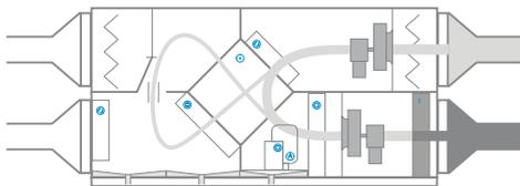
**Dehumidification in the setback mode** is ensured by the heat pump evaporator in combination with pre-cooling in a highly efficient heat recovery exchanger.
