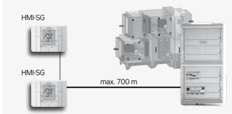
**Figure 22** – Wiring box installation
