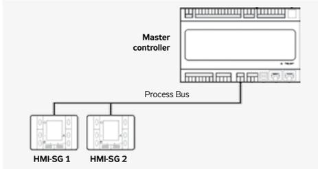
The controller can be installed using a wall wiring box or embedded in plaster. The maximum distance between the control unit and room controller is up to 700 m. HMI-SG controllers are connected to the master controller in series and wiring is always performed to one point.
