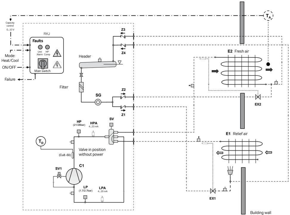
Note: The 4-way valve is displayed in the "cooling" position (SV without power); the E1 heat-exchanger is in evaporator mode.
