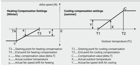
**Figure 13 – Set-Point Compensation (Shift)**
