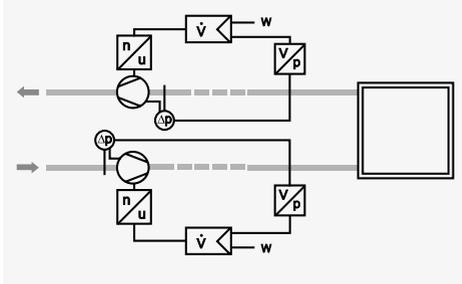
Example: K-factor = 308, Maximum sensor range Pmax = 2000 Pa, Vmax = 13774 m<sup>3</sup>/h. This value is then entered as the maximum range of the sensor in the VCS using HMI.
