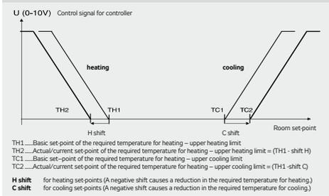
**Figure 12 – Fan Speed Compensation Description**
