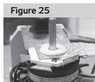
◀ This figure shows blocking of the output stage **1**. The rotary switch can be turned right or left so all stages except stage **1** are available.
