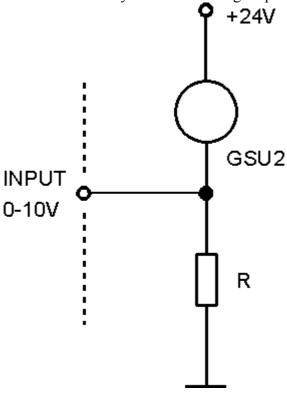
Calculate resistor value with help of Ohm's law. For 0 - 10 V input will fit resistor 500 Ohm e.g. (Parallel combination of 2 pcs 1 kOhm). Don't forget that voltage drop is on the resistor in this case.
