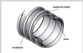
GeoFlex Exhaust HT650 is a high temperature hose designed for extraction or air supply of hot air, fumes, smoke or dust within the industry. Suitable for extraction of exhaust gasses from big combines or excavator etc., or extraction of air from a heater.
