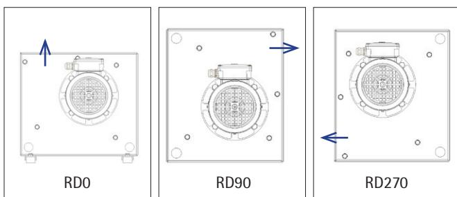
↑ Exhaust air seen from the motor side
