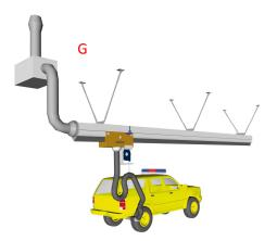
The system sucks out the exhaust gases when you start the motor and during the entrance and exit of the building.
