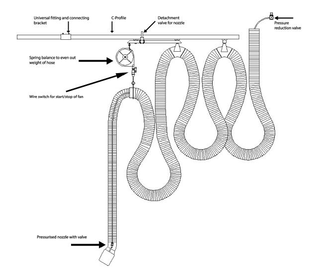
Geovent Festoon system based on a rail system that automatically disconnected from the exhaust when the vehicle leaves the stabling or workshop workplace.
