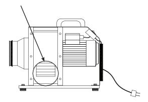
The actual ampere consumption and the kW of the motor are shown on the metal sign on the fan.
