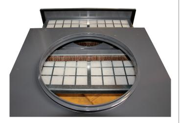
The filter mat is mounted in a retractable filter drawer. When the drawer is pulled out, the filter is cleaned by a built-in brush system. Then the dust may be emptied into a dustbin or a bucket via the drawer.
