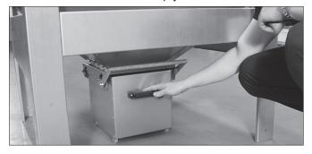
3. Roll bucket in and push handle down while holding bucket in place.
