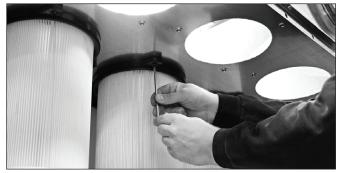
3. Loosen all screws holding the filter cartridge in place.
