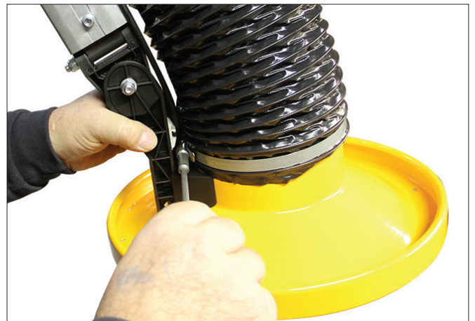
5. Firstly Install the rubber bands, then tighten the band clamp so that the hose is properly secured to the hood. Afterwards place the rubber band over the hose and band clamp.
