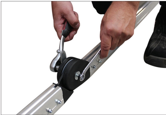
2. The center joint of the arm is attached by tightening the bolt and nut before clicking the gas damper into place.
