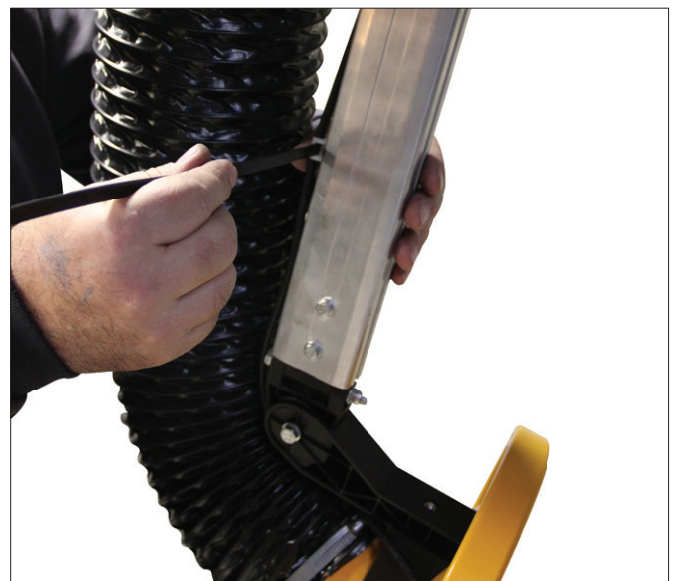
6. Before the hose is installed onto the arm, it is important that the hood is in the position, where the hose is stretched the most. Afterwards place the cable tie inside the retainer and tighten it gently.
