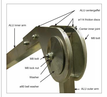
4. Mount the funnel on the outer joint by taking the supplied M8 bolt through 3 disc springs, the alu half, the friction disc, the other alu half and the 3 disc springs and fasten them with an M8 lock nut.
