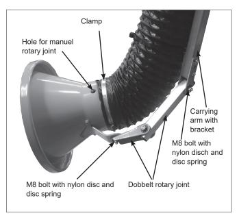
5. The hose is mounted on the funnel by tightening the clamp around the funnel and the hose. Now pull out the hose to max. so that the least possible resistance is left in the hose and fasten with the enclosed plastic binders. Subsequently, the hose is mounted on the branch pipe by means of the clamp.
