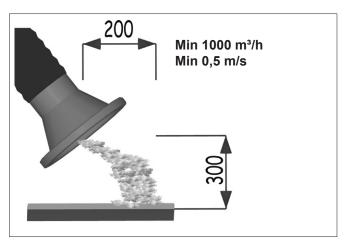
Always check that the correct volume of air is extracted by the suction head/funnel.
