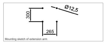
At 4 meters, every joint is assembled and then the Arm is mounted. Next, the spiro pipe is fastened to the extension arm by means of the enclosed self-cutting screws. The part between the spiro pipes is assembled by means of clamps and the supplied hose.
