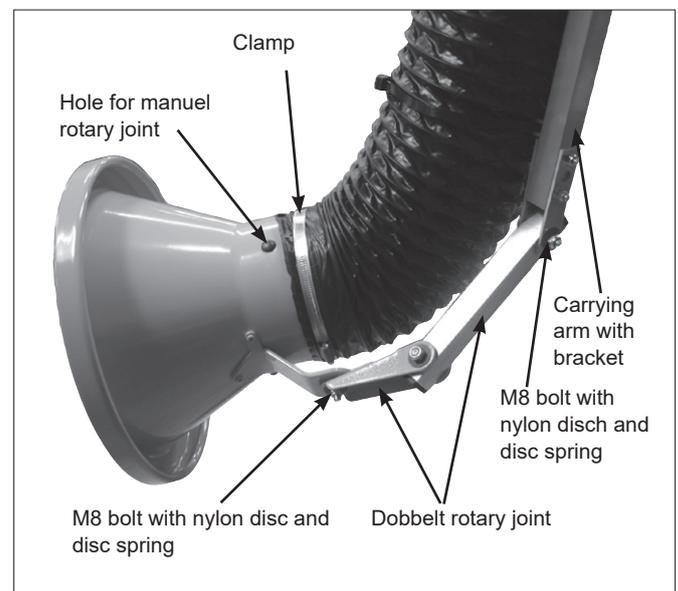
5. The hose is mounted on the funnel by tightening the clamp around the funnel and the hose. Now pull out the hose to max. so that the least possible resistance is left in the hose and fasten with the enclosed plastic binders. Subsequently, the hose is mounted on the branch pipe by means of the clamp.
