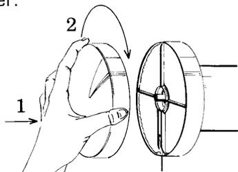
To get access to the filter press the cover and turn it clockwise. Pull off the cover and remove the filter holder. The filter is now accessible to be washed/replaced.
