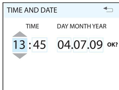
If several values can be changed, the cursor jumps to the right when a selection is confirmed with button 4. The procedure is repeated until all values have been changed to the desired values.
