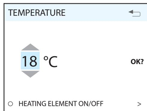
We recommend adjusting the temperature to max 18° so that the air is mixed optimally with the air already in the building.
