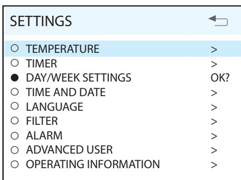
If you select a function that has numerical values, the current value is displayed with a light blue cursor. The value is changed with buttons 1 and 3 and is then confirmed by pressing button 4.
