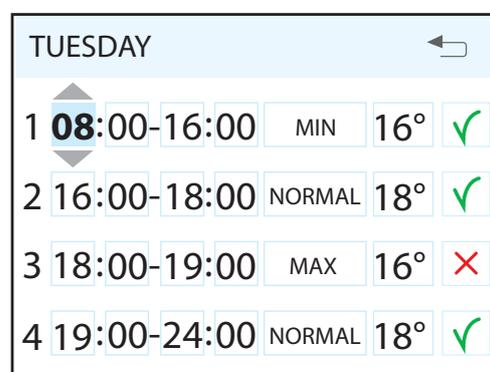
Each day can be programmed with four different time intervals. Adjust the start and stop times for each interval and then adjust the desired speed and temperature. To activate the interval, select a green tick. A red cross means that the interval is not activated. If necessary, then select another interval and repeat the procedure.
