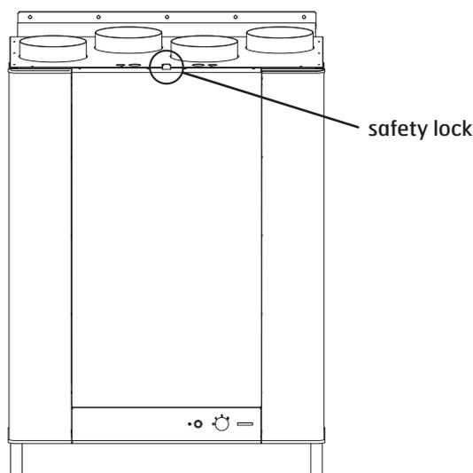
Remember that the door is heavy (10 kg) when lifting it off the unit.
