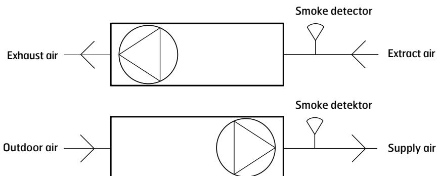
Principal drawing, connection to air handling unit
