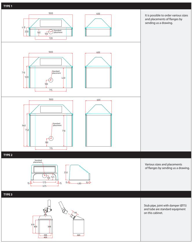
The cabinets are delivered with standard placement of flange unless a special placement is ordered. (all measurements in mm)
