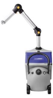
Easy operation with filter saturation indicator and stepless control of volume flow rate.
